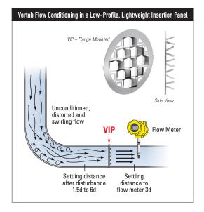
**San Marcos, CA**—A breakthrough, patentpending flat panel flow conditioner, <u>Model VIP</u>, has been introduced by the Vortab<sup>®</sup> Company. This revolutionary flow conditioner maximizes flow meter performance with minimal pressure drop in a simple to install, lightweight thin panel.
