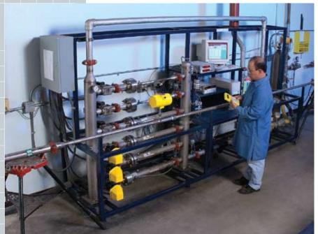
More than 16 precision flow stands to match fluids, fluid conditions, flow rates and line sizes with your application.
